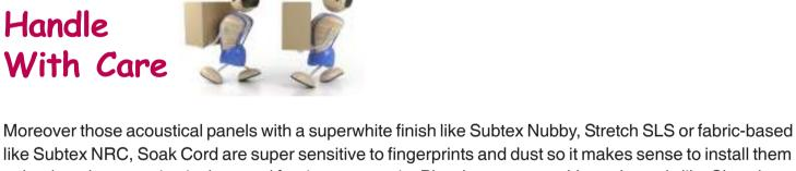
only when the carpeting is done and furniture comes in. Plus there are wood-based panels like Slats that are super sensitive to high humidity and dampness. Again makes sense to install CC18 and SynthPF while waiting out for others to finish before Slats are fixed.
